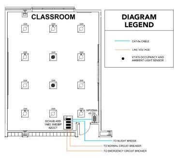
■ Sensors Embedded within Luminaires and nLight Controls
